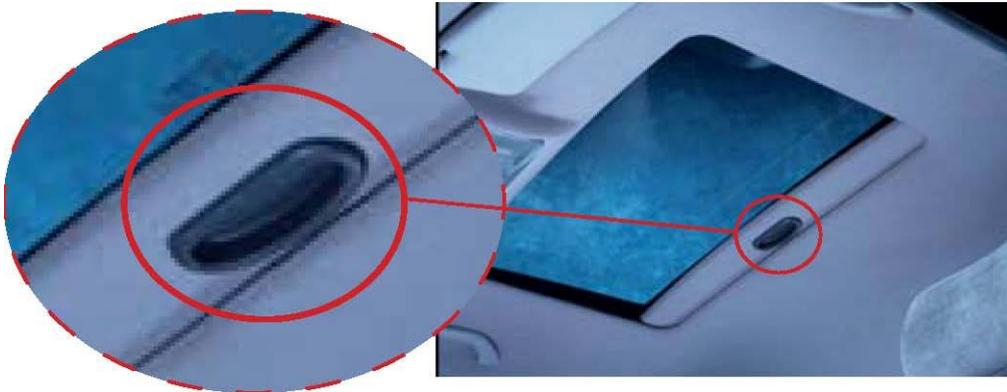
Now with the glass fully open please stick your head up into the opening while looking forward in the vehicle and locate the serial number label. The label is black and white and should be located either in the center or the passenger's side of the vehicle. Next, look at the white part of the label for a bold large black number. This is your sunroof serial number.
